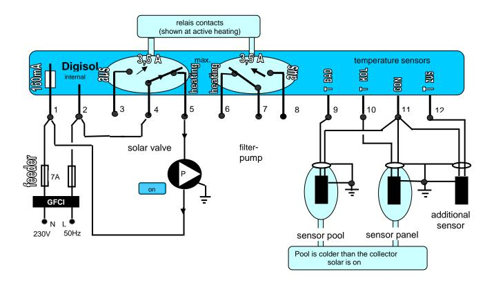
In this example, the collector sensor is warmer than the bath sensor  $\Rightarrow$  the DIGISOL switches on. The bolts show how the current flows over the filter pump and solar pump.
