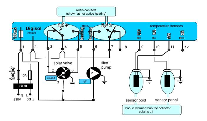
The bolts show how the electricity flows over the motor valve to close it. The pump does not receive any electricity. When the DIGISOL switches on the relay contacts move to the other side. PThe pump runs and the motor valve opens.
