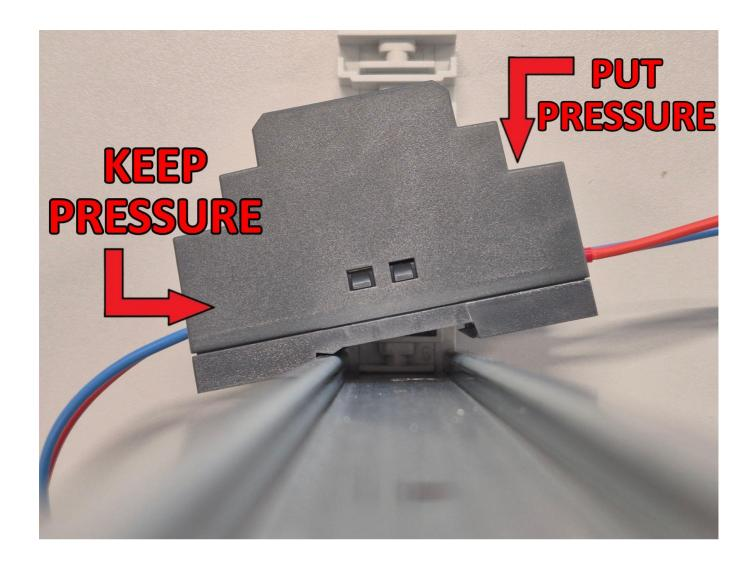
Hook the top on the lip of the rail, while keeping the top side pressed against DIN rail put pressure on bottom of the power supply until audible click sound can be heard.
