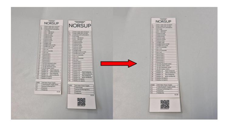
New label is designed to be placed on top of old one with already applied adhesive.
