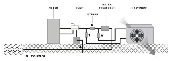
If your installation is equipped of the water treatment with product adductions (e.g. chlorine, brominates, salt...) the by-pass must be installed before the water treatment, with a non-return valve between the by-pass and water treatment.
