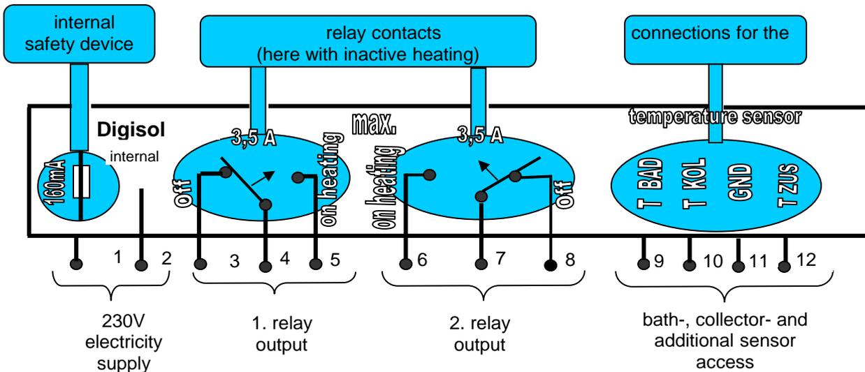
Explanation: A relay is a kind of switch. This “switch” in the DIGISOL is not manually operated like a light switch, but from the DIGISOL itself. In the upper picture you see the relay contacts position with switched off solar heating. Contacts are shown in the neutral position.
