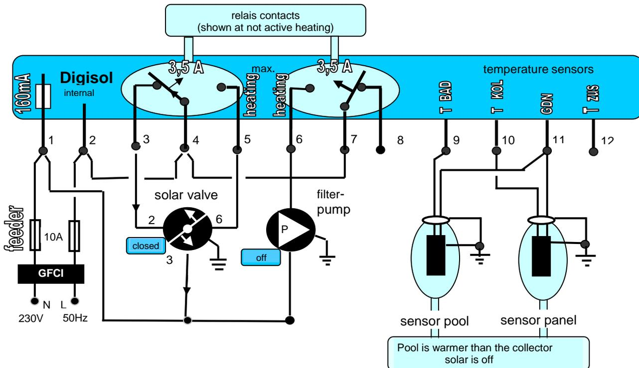
The bolts show how the electricity flows over the motor valve to close it. The pump does not receive any electricity. When the DIGISOL switches on the relay contacts move to the other side. BThe pump runs and the motor valve opens.
