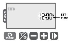
▶ Press + or - to set the hour (ensure that AM/PM setting is correct); then press
