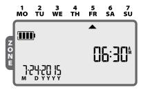
In **AUTO RUN** mode, the ESP-9V will irrigate each zone per its programmed schedule. If any zones are scheduled to run at the same time and day, your controller will place those zones in a queue and irrigate one valve at a time, starting with the lowered numbered zone first.
