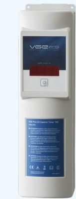
The Control Timer has a LED display for showing the operational lamp hours. The maximum number of burning hours are displayed when the system is started. After this the display counts down to 0, at which time the lamp must be replaced.
