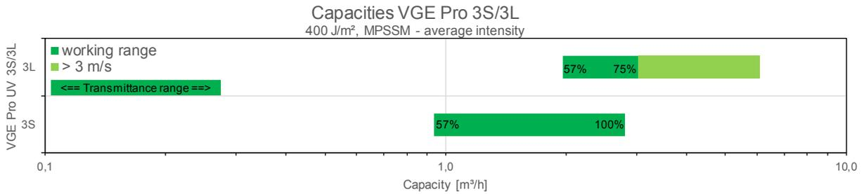
An UV-C dose of 400 J/m<sup>2</sup> equals 40 mJ/cm<sup>2</sup> and the transmittance of the water is measured with UV-C light (254 nm) through 10 mm of water.
