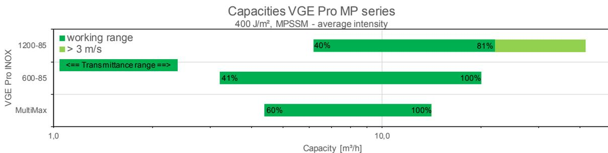
An UV-C dose of 400 J/m<sup>2</sup> equals 40 mJ/cm<sup>2</sup> and the transmittance of the water is measured with UV-C light (254 nm) through 10 mm of water.
