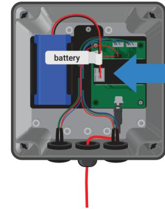
2 Close the Data logger by tightening the screws.
