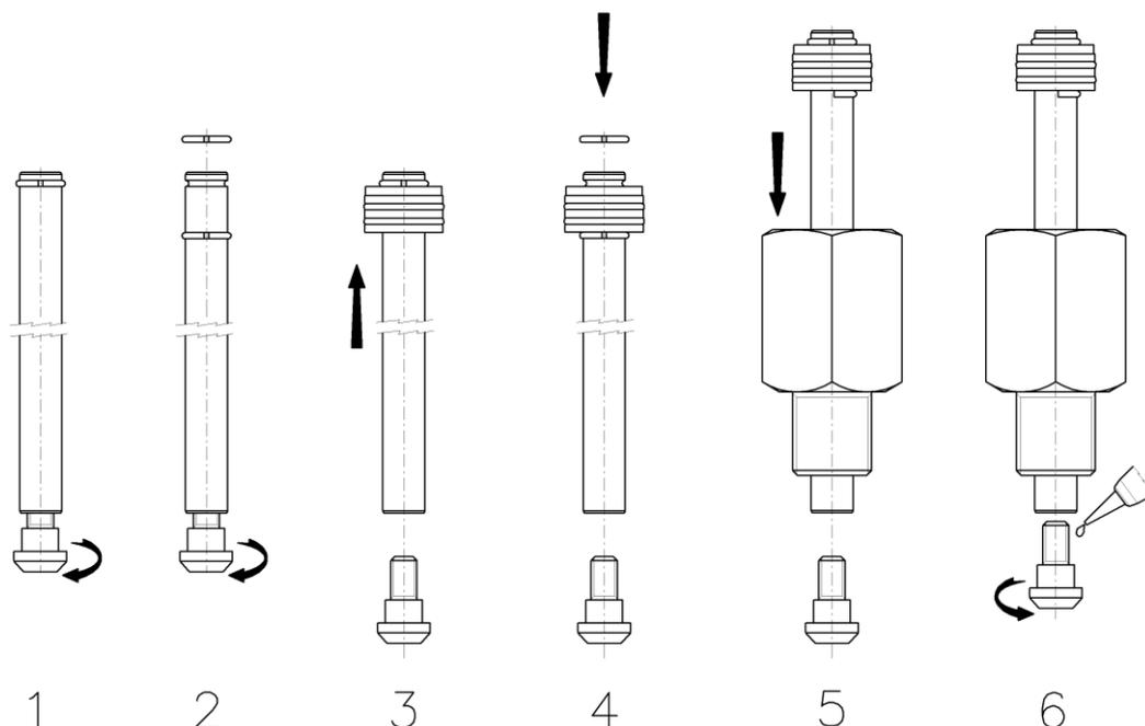
The stem of the cylinders items 0500 – 0510 – 0550 - 0551 is made by two pieces (stem + terminal) and, as a spare part, it is supplied with a pre-assembled stop ring to facilitate the replacing procedure.
