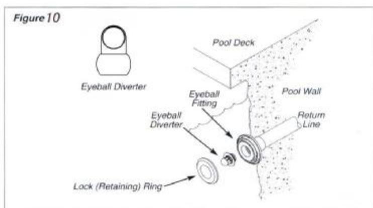
Position the diverter opening to redirect the return line water flow so it does not interfere with the cleaner's movement. Try different positions to see which works best in your pool:
