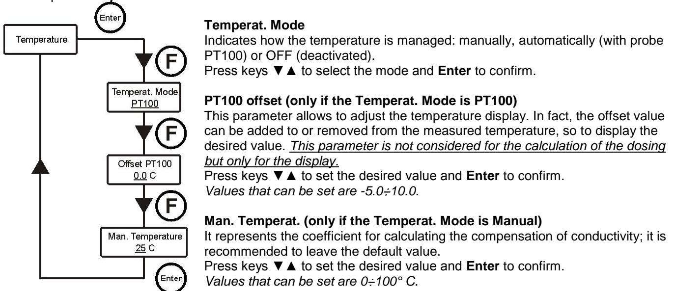
To confirm and exit, press key **Enter** for 3 seconds.
