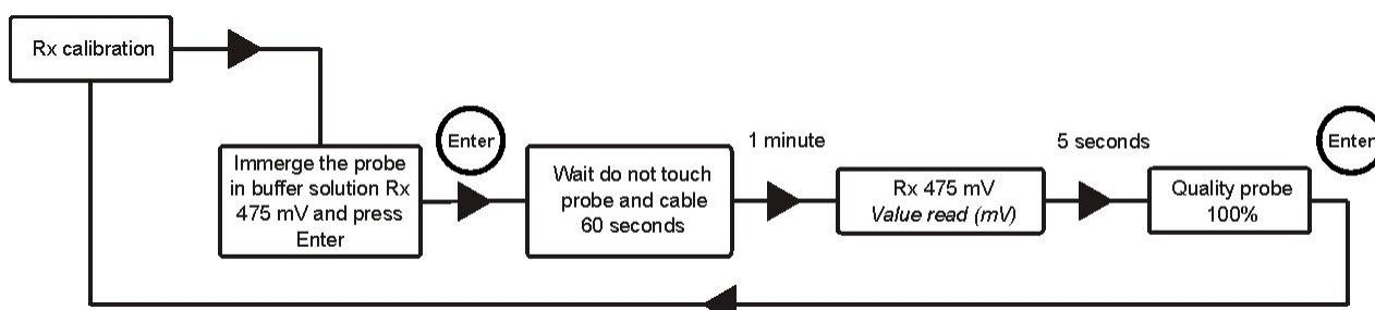
Once the procedure is completed, the quality of the calibrated electrode will be displayed; if the quality of the probe results 25% or less, carry out a new calibration.
