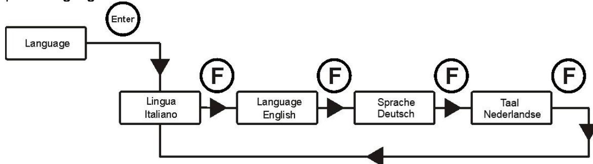
To confirm and exit, press key **Enter** for 3 seconds.
