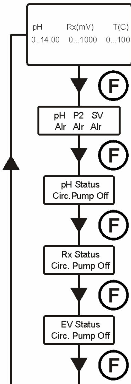
Default screen shows the reading of the pH, Rx and the temperature.
