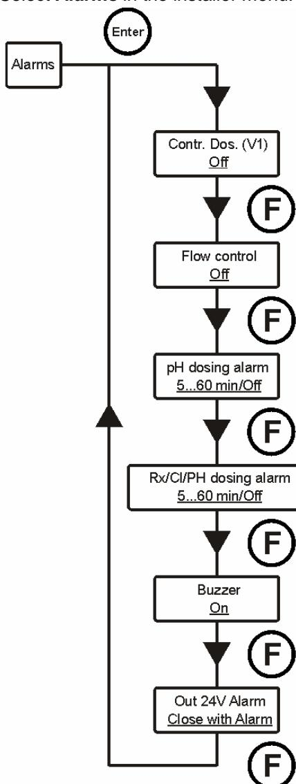
**Contr. Dos. (V1)**. Enables or disables the dosing, when signal V1 occurs (signal of the active recirculation pump). Press keys  $\blacktriangledown \blacktriangle$  to select the two options and **Enter** to confirm.
