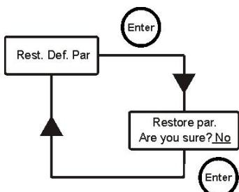
The restoration of the factory parameters is enabled (refer to appendix 1). The system asks if you are sure to proceed.
