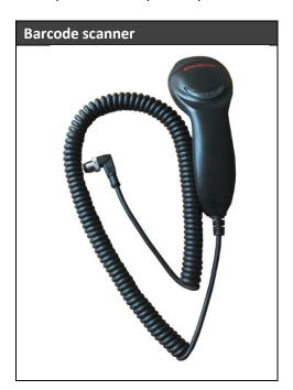
Incorrectly printed or slightly damaged barcodes can be read by placing the scanner directly over the barcode, and then, with the read button pressed, slide the scanner over the barcode. When the barcode is correctly read, the device will emit a sound signal and the screen will display information about the decoded welding parameters.
