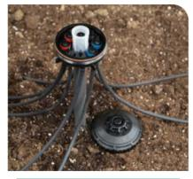
Each port can be configured on the Xeri-Bird™ by installing flow controlled emitters. Above shows a combination of 0.5, 1.0, and 2.0 gph Xeri-Bug emitters.
