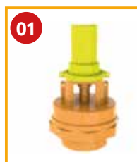
Vacuum Relief Valve 1 1/2 Code 5100200012 Setting range: -0,3 bar / -0,8 bar Working temperature: -20°C / +90°C Thread: G 1 1/2 Weight: 0,65 kg
