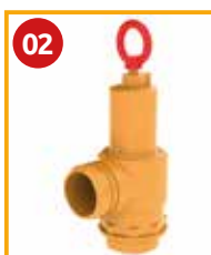
Overpressure Safety Valve - 1 1/4 Code 5100200009 Setting range: +0,3 bar / +1,5 bar Working temperature: -20°C / +90°C Thread: G 1 1/4 Weight: 0,94 kg
