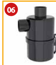
Overpressure Safety Valve 1 1/2 Code 5100200010 Setting range: +0,3 bar / +1,5 bar Working temperature: -20°C / +90°C Thread: G 1 1/2 Weight: 1,02 kg
