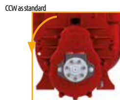
Version HM MEC9000: 100 cc/rev Pmax 175 bar - In G 1/2" - Out G 1/2" MEC11000: 125.7 cc/rev Pmax 175 bar - In G 1/2" - Out G 1/2"
