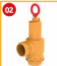
Overpressure Safety Valve 1 1/2 Code 5100200010 Setting range: +0,3 bar / +1,5 bar Working temperature: -20°C / +90°C Thread: G 1 1/2 Weight: 1,02 kg
