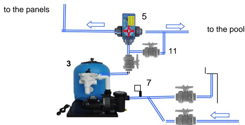
6. Put tee for collector flow line into pipe leading to the pool. Glue stop cock (9) - downdraft brake into flow line pipe.
