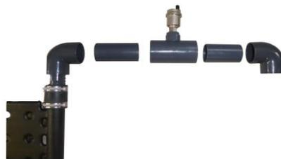
5. Install 3-way valve (5) behind filter pump (3).
