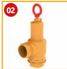
02 Overpressure Safety Valve - 1 1/2 Code 5100200010 Setting range: +0,3 bar / +1,5 bar Working temperature: -20°C / +90°C Thread: G 1 1/2 Weight: 1,02 kg
