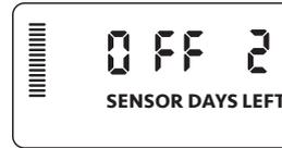
An active Clik Delay can be cancelled by turning the dial to the OFF position, waiting for OFF to stop flashing, then turning the dial back to the RUN position.
