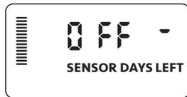
4. Press the “+” button to set Clik Delay duration (from 1 to 7 days).
