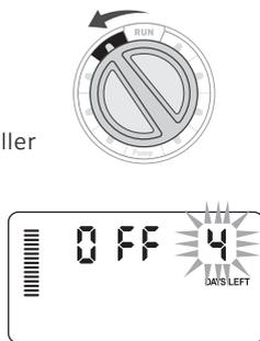
4. Turn the dial back to the **RUN** position, at which time, **OFF**, a number and the **DAYS** icon all remain on.
