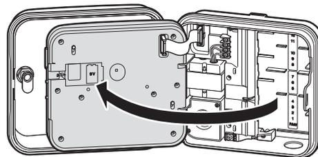
Connect a 9-volt **alkaline** battery (not included) to the battery terminals and place in the battery compartment in the front panel. The battery allows the user to program the controller without AC power. **Watering will not occur without AC power.** Since this controller has non-volatile memory, the program clock and calendar will be retained during a power outage even if no battery is installed.
