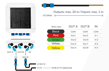
We recommend using resin-filled watertight connectors and terminating unconnected cables with them to prevent oxidation.
